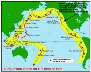
What's known as the "Ring of Fire" accounts for 90 percent of all earthquakes and 81 percent of the world's largest earthquakes. The Cascadia Subduction Zone is part of Ring of Fire and the only significant fault along the ring that hasn't experienced a major earthquake in the past 50 years.
