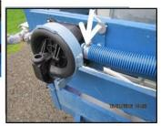
Outlet coupling 1 ½ "reduces clear vinyl tube to 1" with stainless steel clamps
