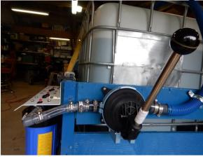
System uses a Gusher Titan BP4402 hand powered bilge pump for operation when electrical power is down. System can be upgraded for electrical pumps when power and pumps become available.
