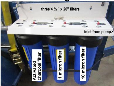
System uses a Triple Big Blue filter housing and bracket (4.5"x20" filter canisters) to improve flow and prolong filter life. The filters are mounted on the passenger side of the trailer to avoid road spray. Each canister is fitted with drain cocks so canisters can be drained before opening. Canisters should be empty for travel. The bungee cord holds the housings against a 2"x6" to prevent vibration during travel. Filters are Big Blue 10 micron, 1 micron and carbon block filters.
