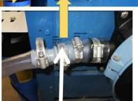
1 ½" skimmer hose fastened to pump with stainless steel clamps
