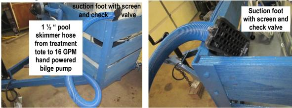
Chlorinated water is drawn from the tote through the suction foot/check valve via a 1  $\frac{1}{2}$ " pool skimmer hose by a 16 GPM hand powered bilge pump. The large diameter skimmer hose provides additional volume to the pump.
