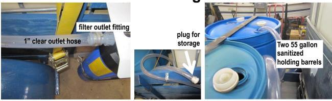
System uses standard PVC fittings and 10 feet of 1" clear outlet hose to convey treated water from the filters to the storage distribution reservoirs. Storage for this unit is 2 each 55 gallon food grade barrels with standard hose bibs.
