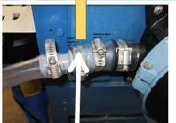
1 ½" skimmer hose fastened to pump with stainless steel clamps
