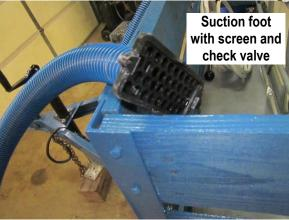
Chlorinated water is drawn from the tote through the suction foot/check valve via a 1  $\frac{1}{2}$ " pool skimmer hose by a 16 GPM hand powered bilge pump. The large diameter skimmer hose provides additional volume to the pump.
