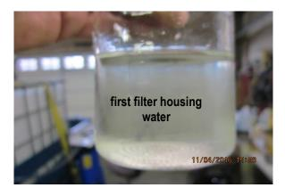
1 micron filter condition after 120 gallons (must meet NSF/ANSI 53 or 58 standard).
