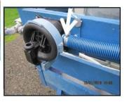
Outlet coupling 1 ½ "reduces clear vinyl tube to 1" with stainless steel clamps
