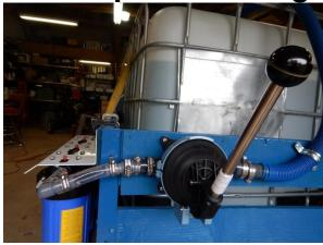
System uses a Gusher Titan BP4402 hand powered bilge pump for operation when electrical power is down. System can be upgraded for electrical pumps when power and pumps become available.
