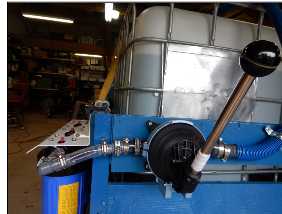
Here is the Titan Gusher 16 GPM hand operated bilge pump with hoses running from the tote to the filters. The pump is capable of 6 to 8 GPM with comfortable operator effort.
