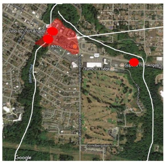
Expect severe liquefaction and compaction failure in fill over White Creek Valley.
